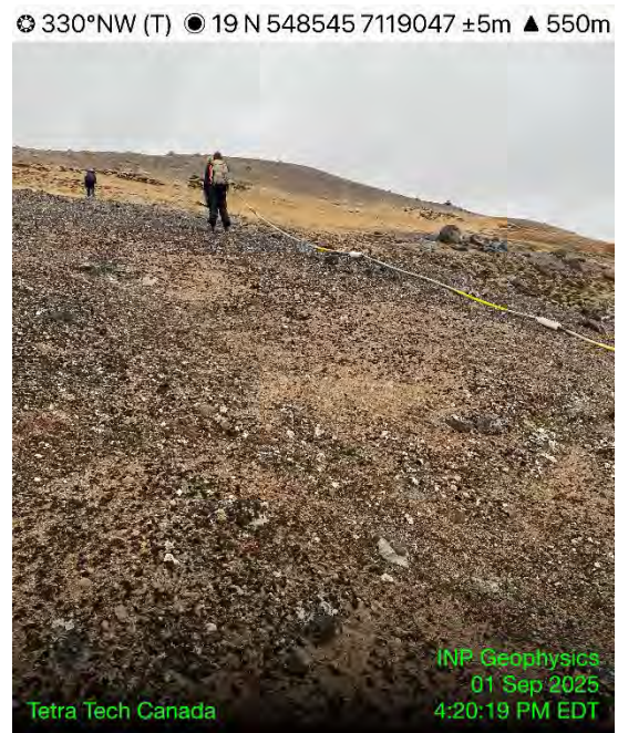
Images 5-2 and 5-3: 50 MHz RTA survey on the East Alignment on Lines X3 (left) and X5 (right) respectively
