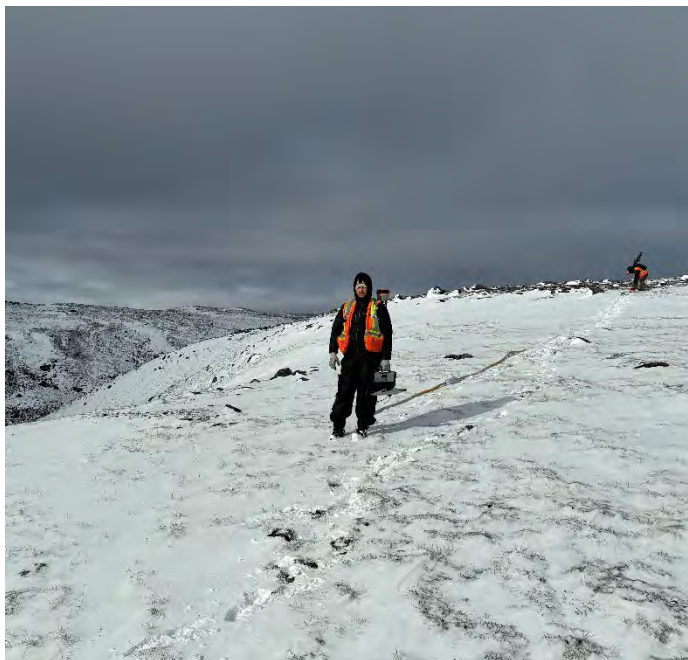
Images 5-2 and 5-3: 50 MHz RTA survey on the East Alignment on Lines X3 (left) and X5 (right) respectively
